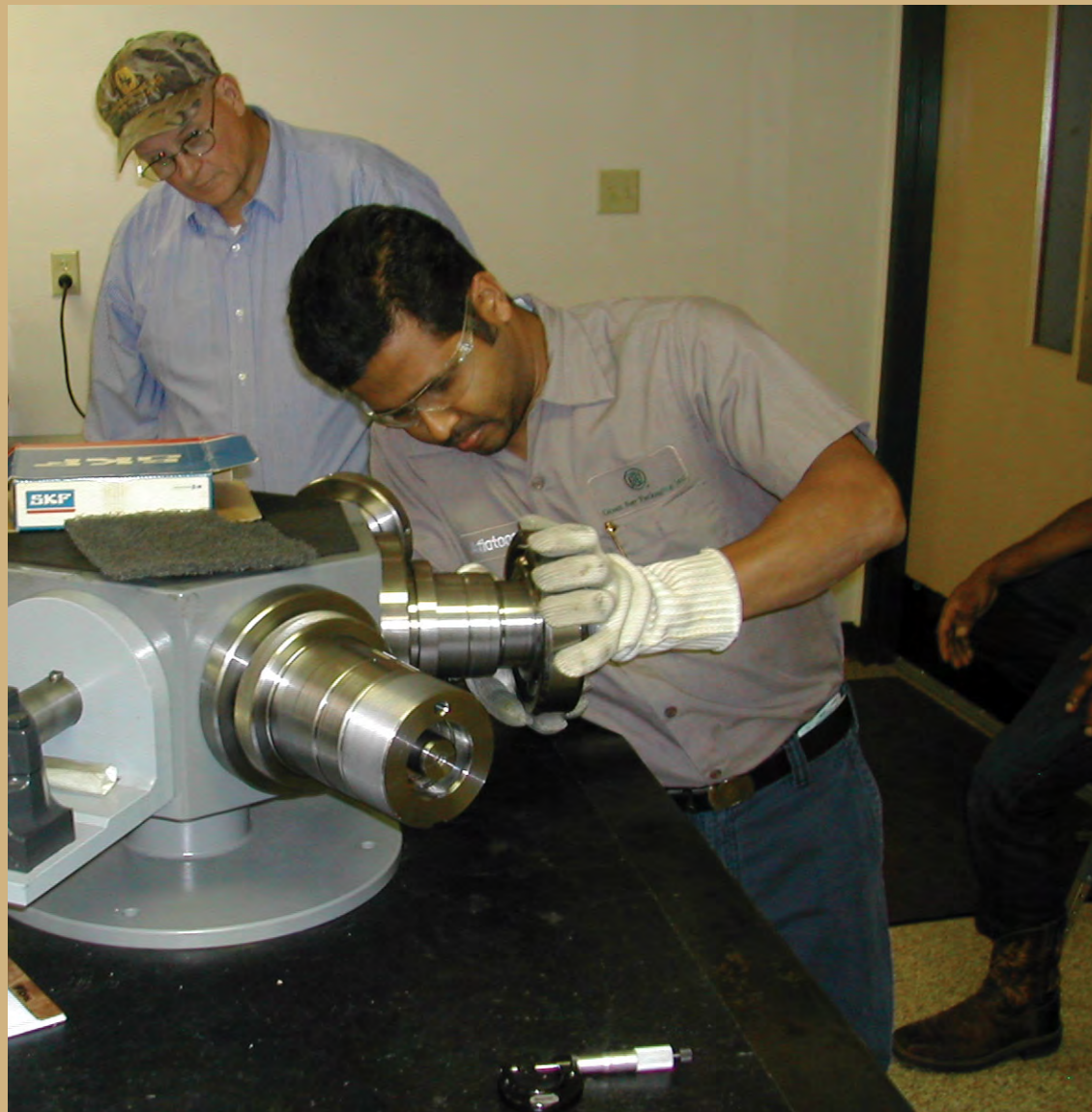
Green Bay Packaging, Inc.-Arkansas Kraft Division - Mechanical Maintenance Instructor Ronnie Halsted (left) looks on as GBP Maintenance Technician Aflatoon Kawsar properly mounts a bearing during Bearing W& Lubrication Training.
